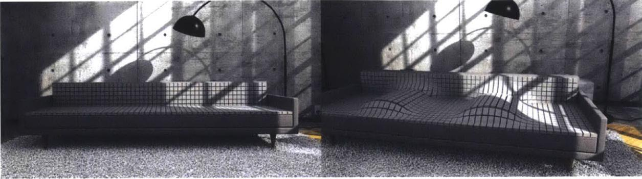
*Figure 74. Exoskin illustration with thick wool felt panels integrated into an elastic layer embedded with an array of actuatable bladders, to form a dynamic soft sofa.*
