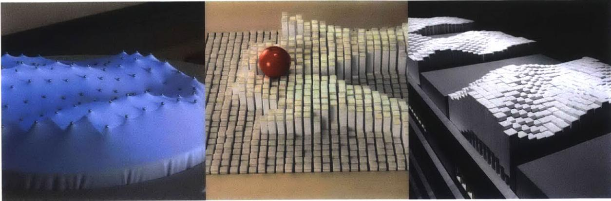
Figure 11. From left to right: (1) Relief: low-density shape display with latex sheet covering, (2) inForm: higher-density display capable of representing human-scale features, and (3) TRANSFORM: design-lead piece able using motion to depict waves & other non-rigid modalities
