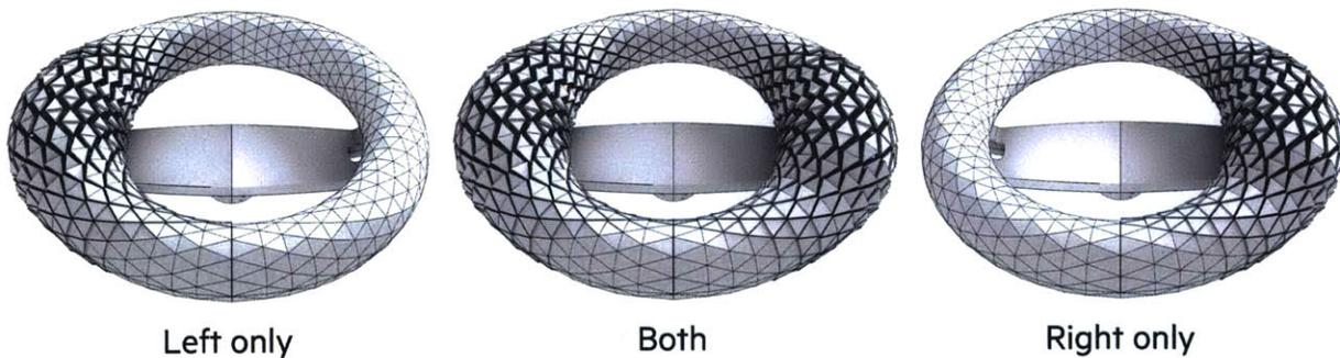
Figure 63. Larger deformations using the bulky air bladders nearest the bottom create an alarming and uniform inflation for alerting drivers of danger, pedestrians, and other potential collision hazards.
