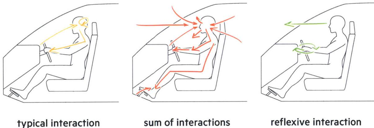
Figure 59. Diagram showing the progression from a typical automotive interaction loop requiring a glance at the dashboard to an evolved reflexive interaction loop allowing the hands to bypass the eyes.
