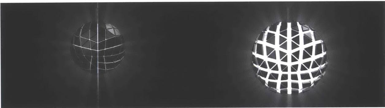
Figure 71. Illustration of opaque Exoskin rigid material with interior light source and dense panelization method in order to create a dimmable lamp. Left shows the default state while Right shows the inflated, actuated state.
