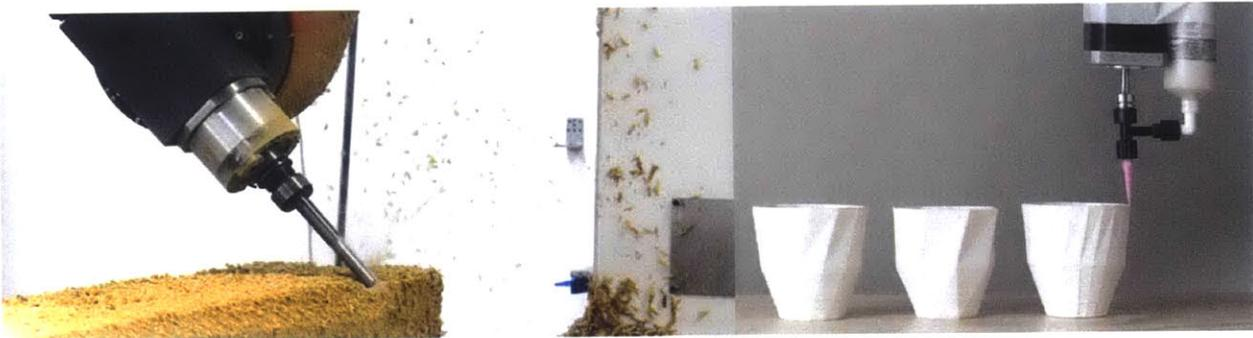
Figure 27. Left: 5-axis CNC milling of a wooden block using a KUKA Robotics arm to create a complex form. Right: Antwerp-based design studio Unfold 3D printing ceramic using their proprietary method.
