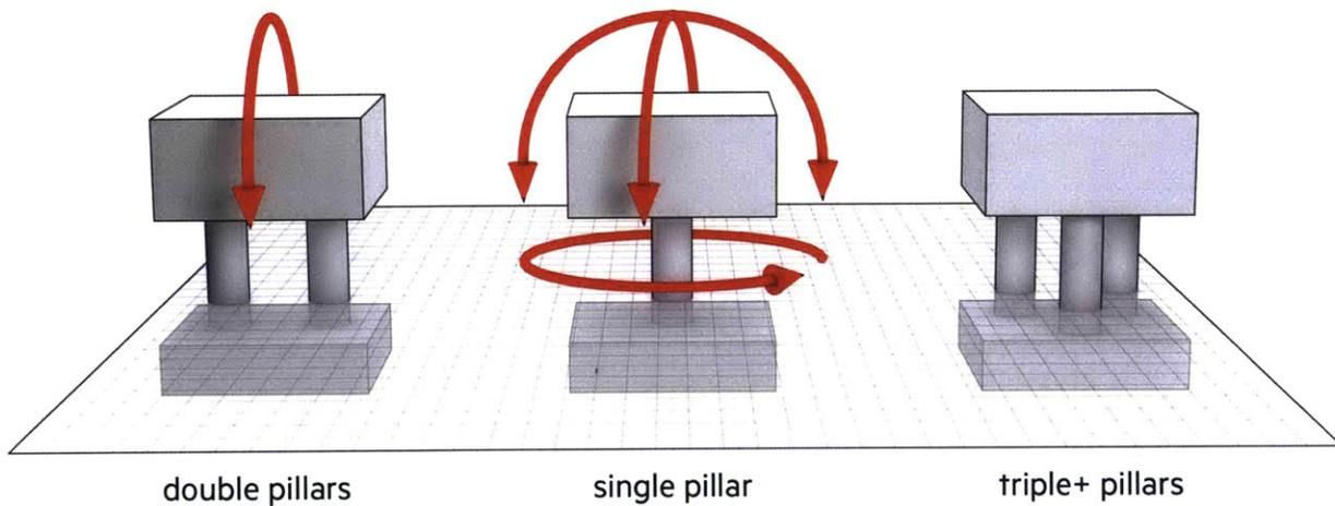
Figure 44. Illustration showing the degrees of freedom of movement for an individual rigid scale depending on the number of pillars.
