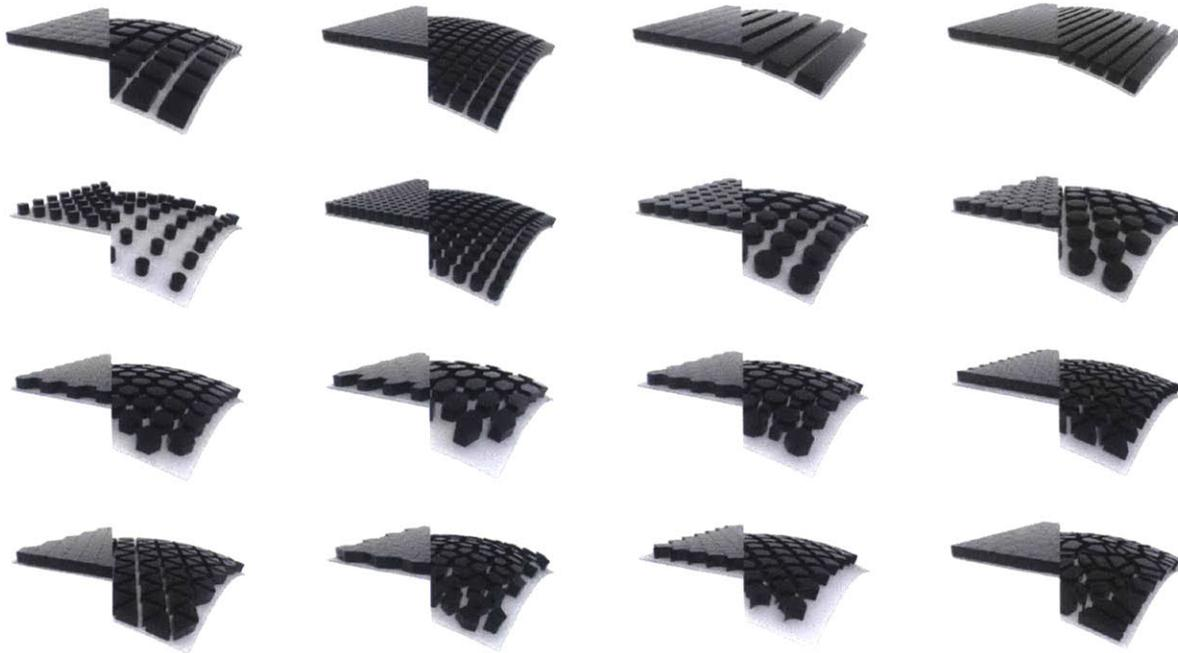
Figure 31. 3D visualization of the panelization methods from Figure 30 including quad meshing, triangular, hexagonal, voronoi, and more. Shown here are the default and actuated states of each.
