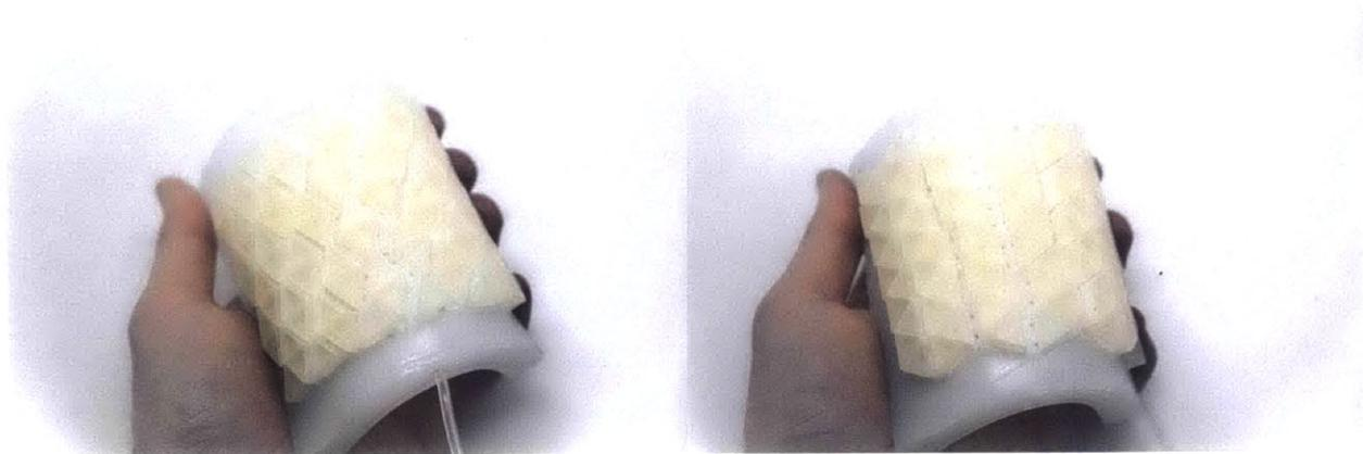
Figure 50. Anisotropy seen in deformation. Flexure in the Y axis caused the scales to group like diamonds (Left) while flexure in the Z axis caused them to group in rows (Right).
