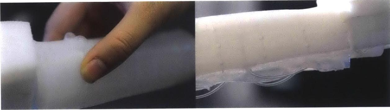
*Figure 18. Over-actuated smaller air bladders in top layer in order to better show the tactile shape change happening underneath the palms during GPS turn navigation*
