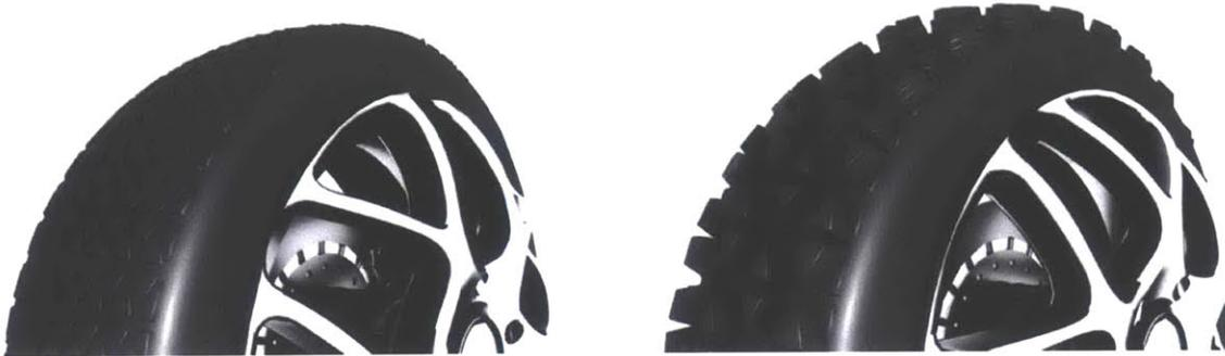
*Figure 72. Exoskin composite illustration of thick rubber scales used to actuate high-pressure inflatable air bladders that improve traction and stability. Left shows the default state while Right shows the actuated state.*
