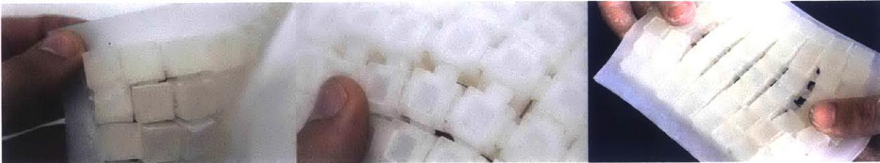
*Figure 45. Exoskin composite prototype photographs showing the thin silicone connective tissues in-between the scales.*
