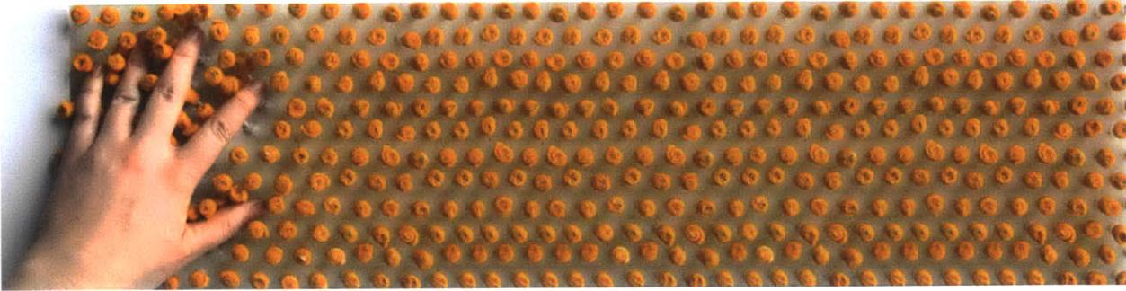
*Figure 10. Super cilia skin is a tangible interface which responds to touch. Like our skin, it is a haptic I/O membrane that can sense and simulate movement and wind flow.*
