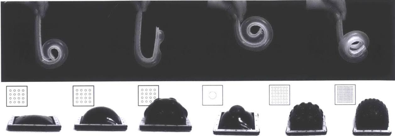
Figure 5. Top: Pneu bending shape primitive. Bottom: shape primitive of multi-stage texture change
