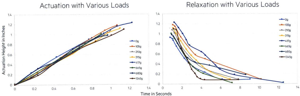
Figure 54. Exoskin composite actuation and relaxation tests under various loads up to about a kilogram.
