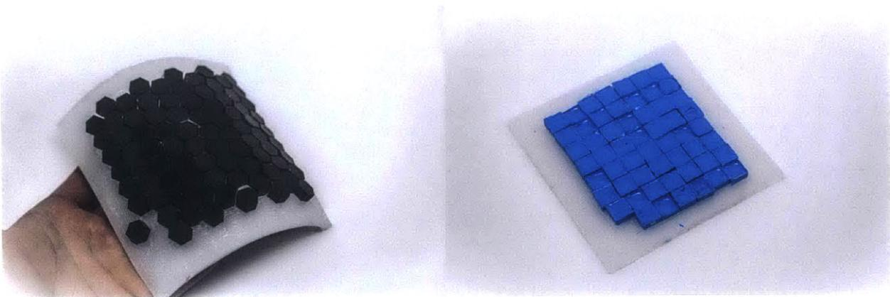
Figure 43. Left: Lasercut acrylic scales epoxied to silicone sheet. Right: Hand-molded urethane-based resin plastic square scales epoxied to silicone sheet.
