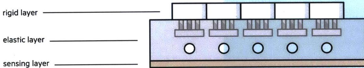
Figure 23. Simplified illustrated diagram showing the three key layers in Exoskin
