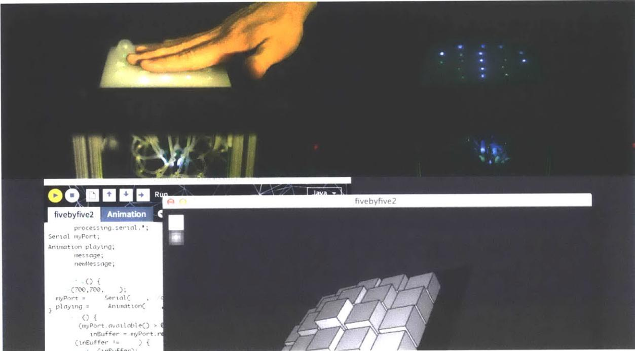
Figure 6. Pneuxel is made of five by five individually controllable cells that can light up through an optical waveguide composite. It can simulate variable degrees of expansion and contraction through pneumatic actuation. Shown here is the device and software implementation.
