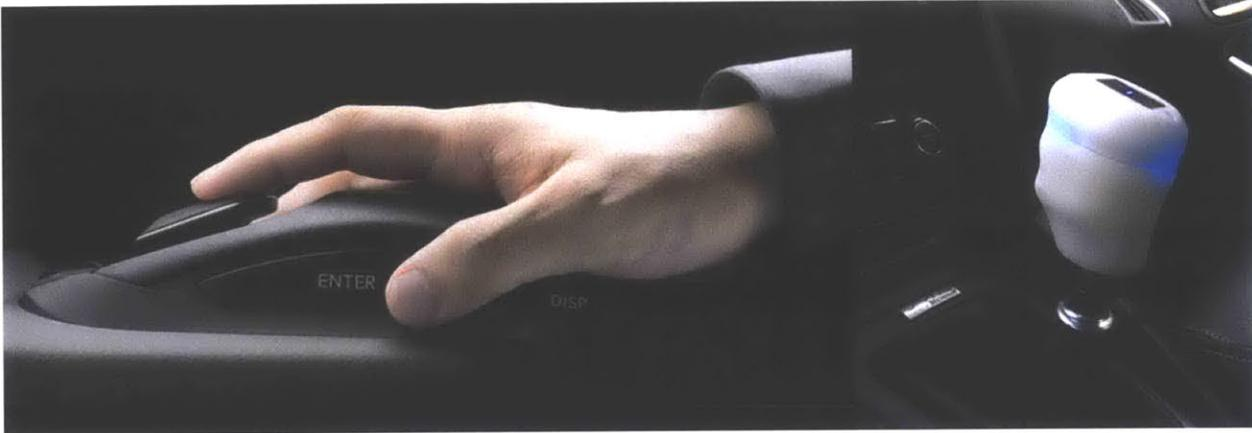
Figure 58. Left: Lexus' haptic Remote Touch Interface touchpad. Right: Haptic Feedback Shift Knob by Zachary Nelson that vibrates when it's time to select another gear.
