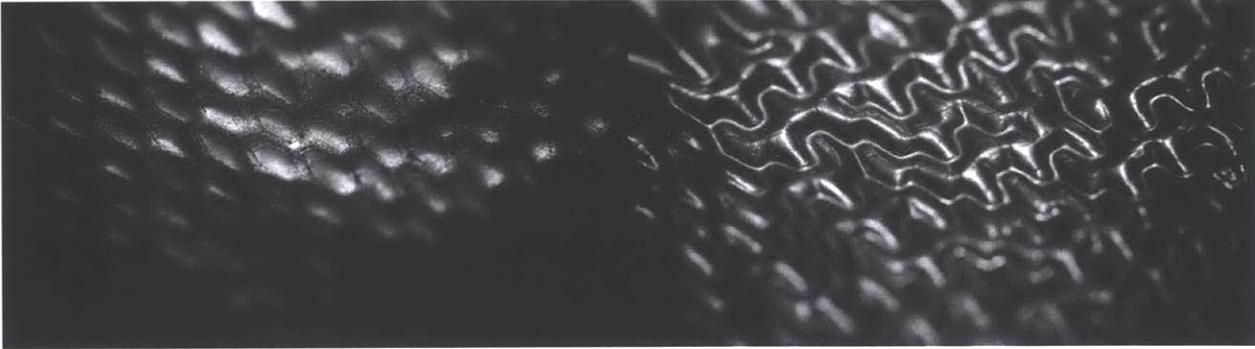
*Figure 22. Macro photographs showing the texture change using the Biologic natto cells on latex. The left photograph shows their humid state, while the right photograph shows the arid state.*
