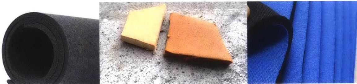
Figure 28. Left: Wool felt. Center: Two pieces of raw leather hide Right: Blue neoprene rubber fabric.
