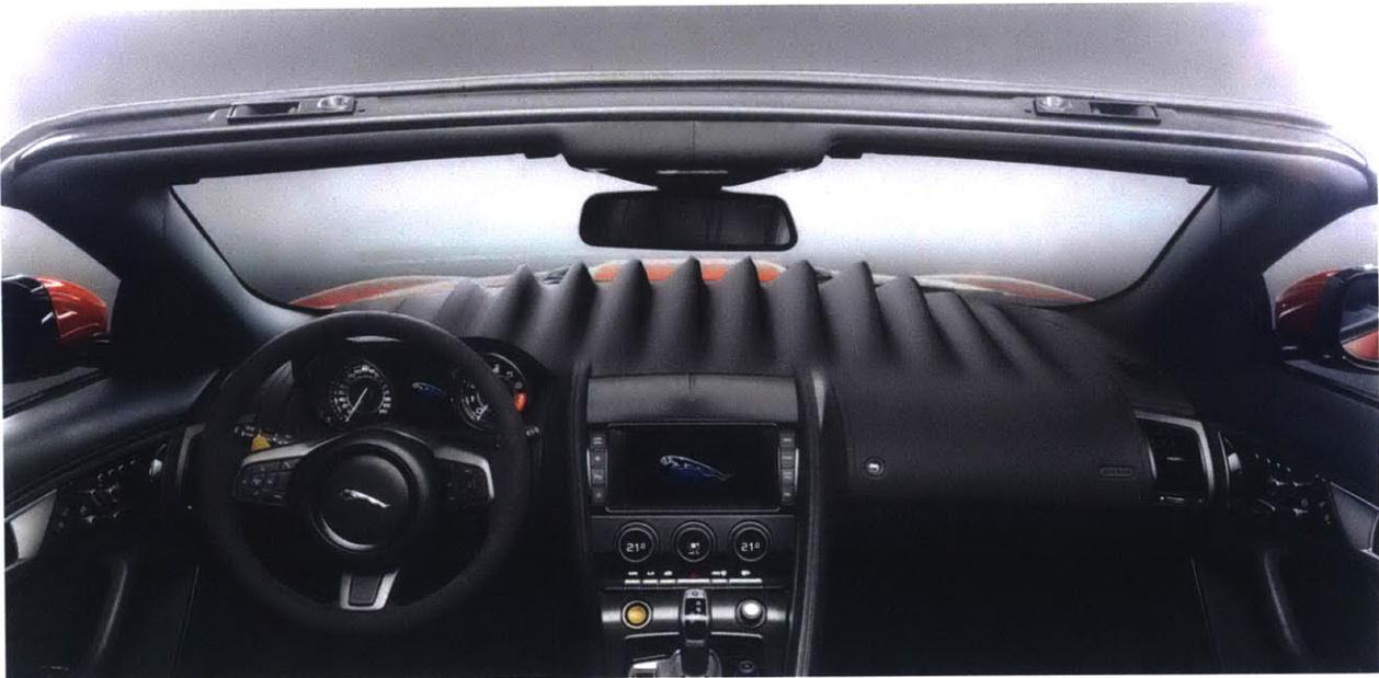
Figure 21. Illustration of the reactive dashboard actuating with the high speed movement of the car
