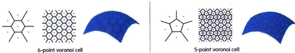
Figure 33. Voronoi cell panelizations on positive curved surfaces by Stavric et al.
