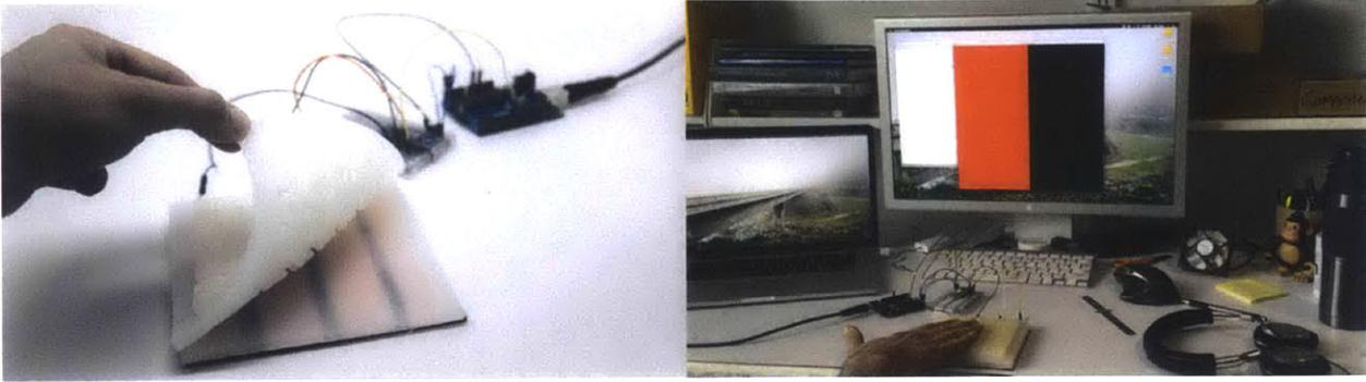
Figure 52. Copper-based capacitive sensing layer prototype with Arduino platform
