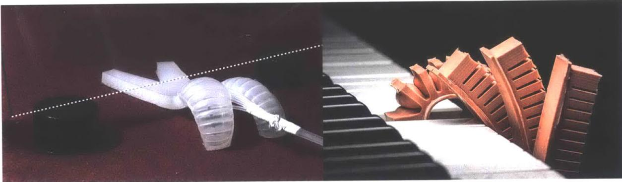
Figure 13. Left: The soft robot can wiggle its way underneath a pane of glass just three-quarters of an inch above the surface. Right: Four soft robotic fingers progressively curl to play notes on a keyboard.
