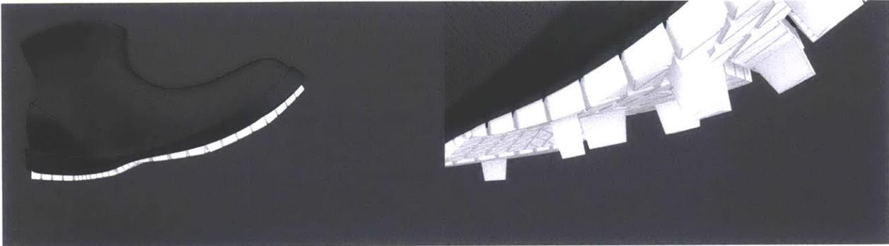
Figure 68. Illustration showing the application of Exoskin as the sole of an active shoe. Left: default state, Right: actuated state.
