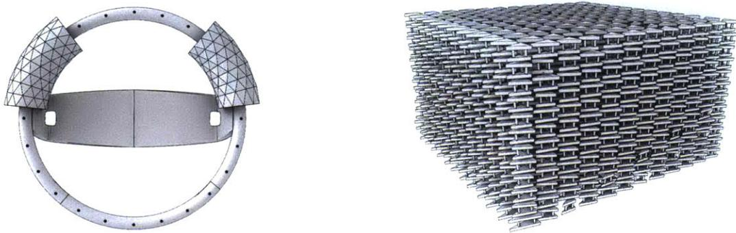
Figure 67. Right: Illustration showing stacked rigid 3d-printed panels ready for fabrication. Left: Those same panels applied to the wheel illustrating the quantities needed to fully cover the surface.
