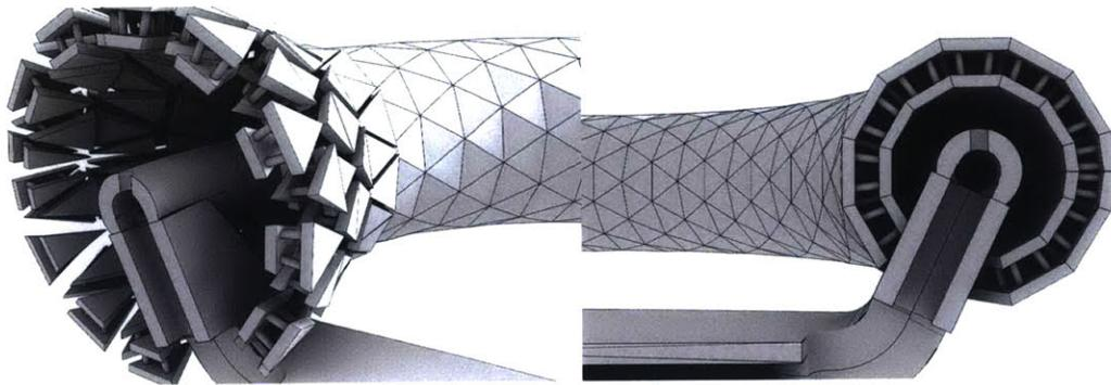
Figure 66. Close-up illustrated views of the molding architecture, panelization, and spoke structure of the prototype design.
