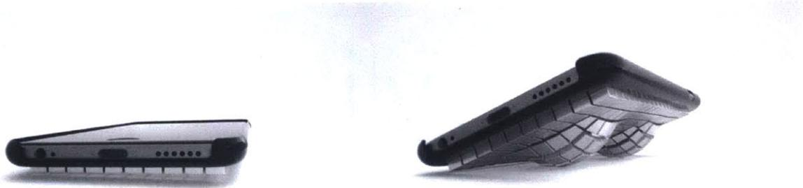
*Figure 70. Illustration showing the application of Exoskin embedded into a mobile phone case. Left: default state, Right: actuated state while watching a video.*
