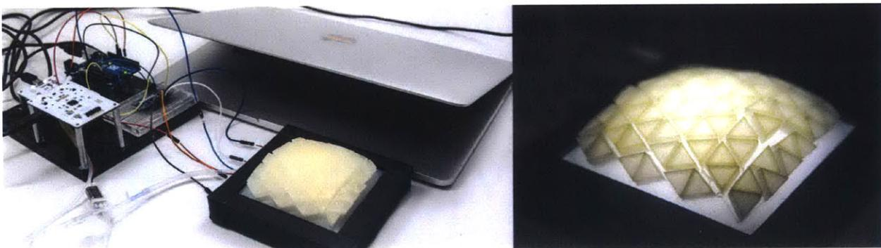
Figure 53. Combined prototype with capacitive sensing, embedded LED, and actuation all on dynamic feedback loop controlled by both an Arduino and Pneuduino.
