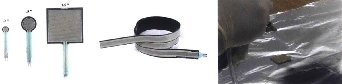
Figure 40. Left: variety of pre-fabricated force resistive sensors available off-the-shelf from sites like Sparkfun and Adafruit. Right: Applying FSR ink to a surface using an airbrushing system.
