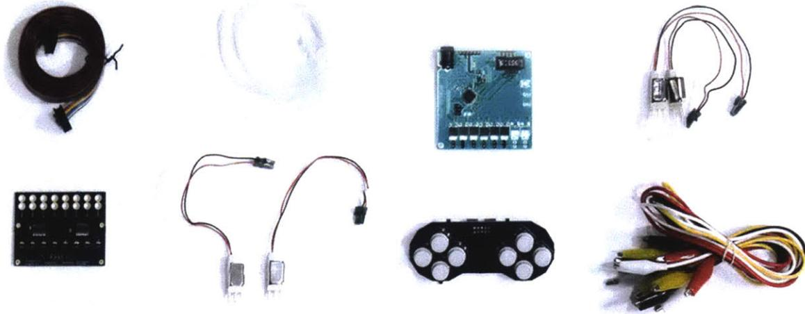
Figure 38. Pneuino prototype system components designed by Felix Heibeck
