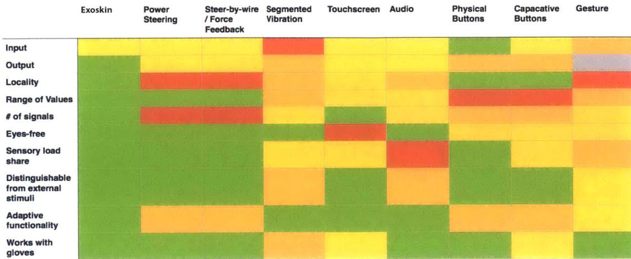
Figure 60. Chart comparing various input and output mechanisms used in automotive steering wheels
