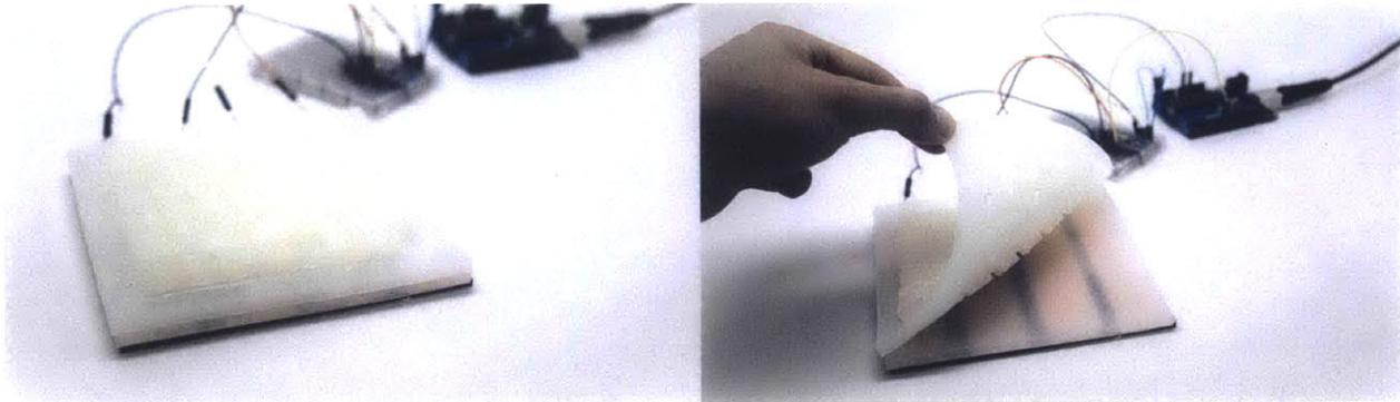
Figure 41. Copper-based capacitive sensing layer prototype with Arduino platform
