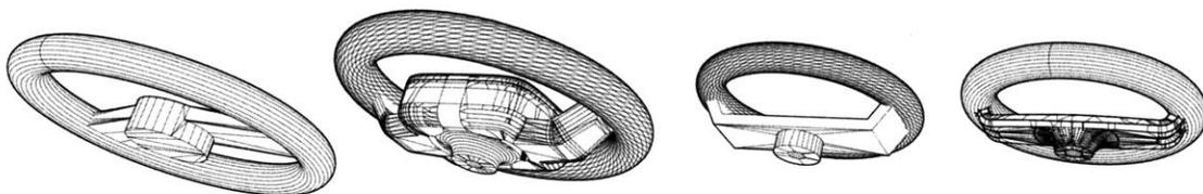
Figure 64. Illustration showing the iterative progression of the designs for Exowheel.
