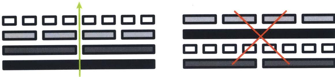
Figure 37. Illustration showing the correct, ascending order for actuated bladders in the elastic layer
