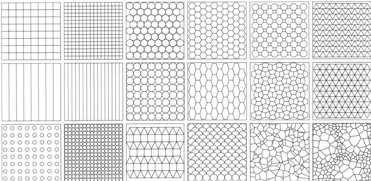
Figure 30. Variety of 2D panelization methods explored in early Exoskin samples including quad meshing, triangular, hexagonal, voronoi, and more.
