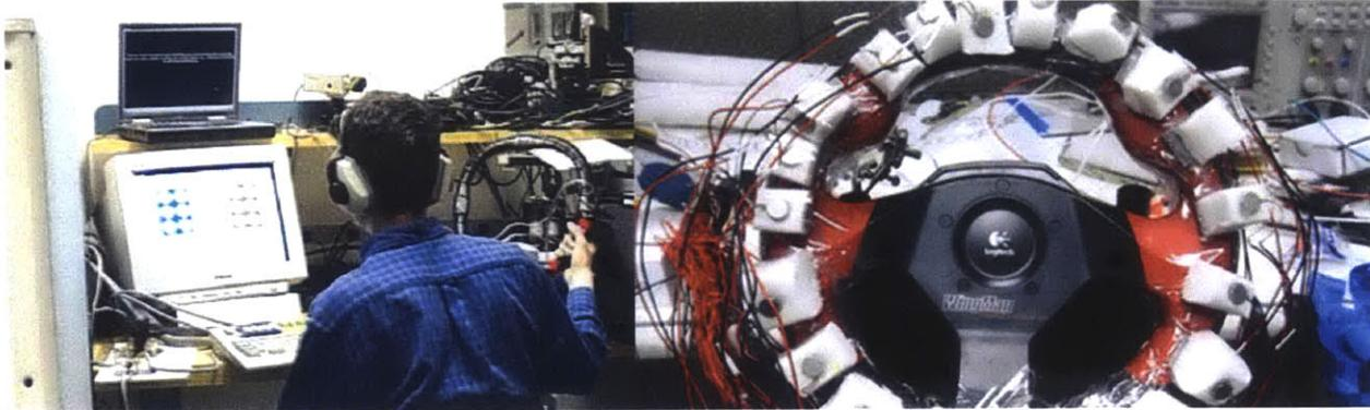
Figure 57. Left: Enriquez's tactile wheel that provides haptic feedback to alert the driver of a possible problem. Right: Haptic steering wheel developed by AT&T using 20 vibration motors.
